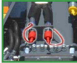
Double acting hydraulic function on the lift arm (mechanically operated)
