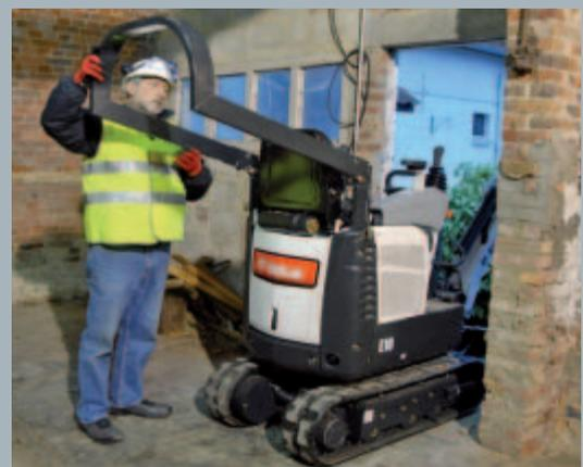
Both models are equipped with a foldable TOPS structure.
