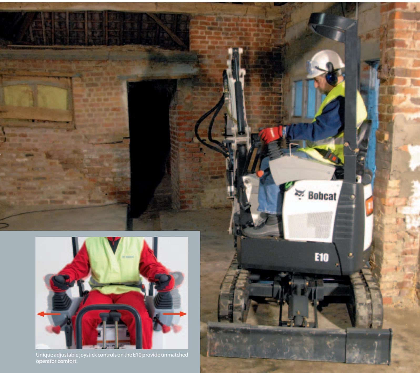
Unique adjustable joystick controls on the E10 provide unmatched operator comfort.
